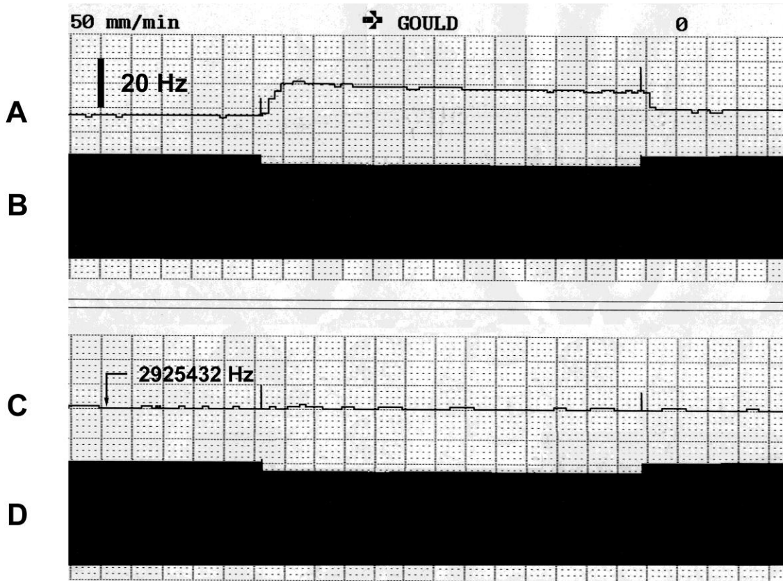
Fig. 2: Effects of power liner voltage changes on PTO frequency A,B with 3TF7 C,D with 3TF7 replacement module
